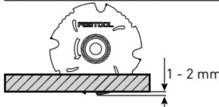
Set the cutting depth according to the workpiece thickness – tooth projection of 1–2 mm.
